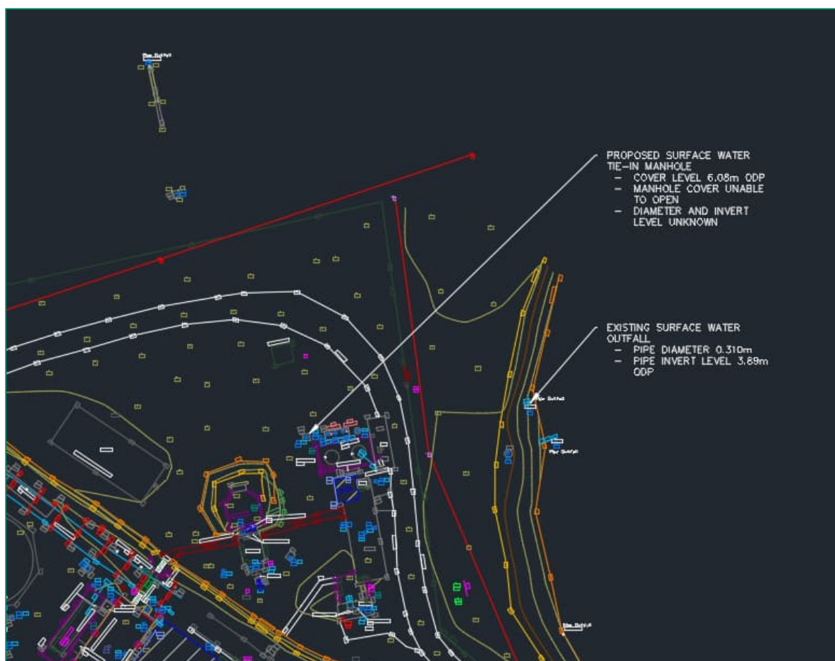
Figure 3-2: Existing Drainage Outfall Locations (Source: Extract from Murphy Geospatial Tarbert Power Station Topographical Survey (Murphy Geospatial DRG no. MGS54284_T_ITM_Rev1_01))
