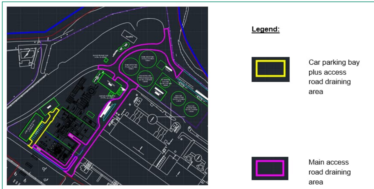
Figure 4-1: An extract of surface water drained area for the proposed bypass oil separators
